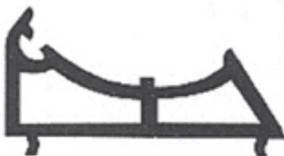
Angled Post Adapting Profile (27.3 x 57 mm)
